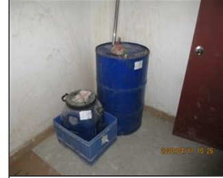
Photo of non-conformity NC-One bucket of cleaning detergent without leaking proof facility.JPG
