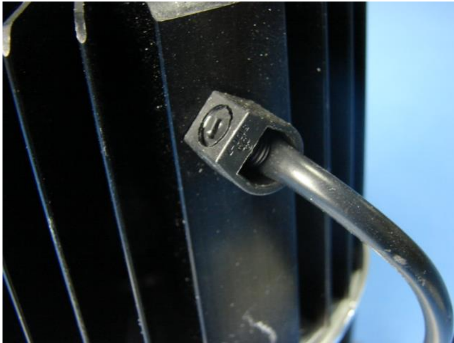
Picture 13: DLC1070-A840 anchorage view
