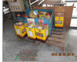
Photo of non-conformity No secondary containment for chemical.JPG
