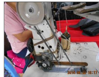
Photo of non-conformity No safety guard for rolling part.JPG
