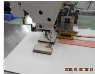
Photo of non-conformity No needle guard was installed.JPG
