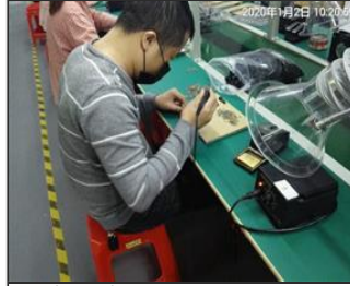
Photo of non-conformity NC-improper PPE wearing.jpg
