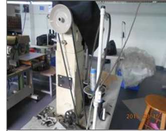
Photo of non-conformity Sewing machine missing pulley guard.JPG
