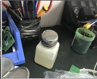
Photo of non-conformity NC - A container with industrial alcohol used at the repairing station not labelled with identification.JPG
