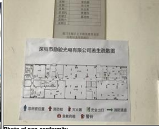
Photo of non-conformity NC - The layout of the posted evacuation plan not matched with the actual layout and no emergency evacuation assembly point identified.JPG
