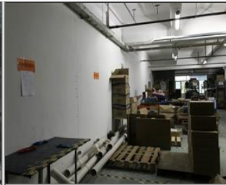
Photo of non-conformity NC - Materials stored against wall.JPG
