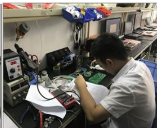
Photo of non-conformity NC - The soldering worker working at the repairing station not provided with dust-proof mask.JPG
