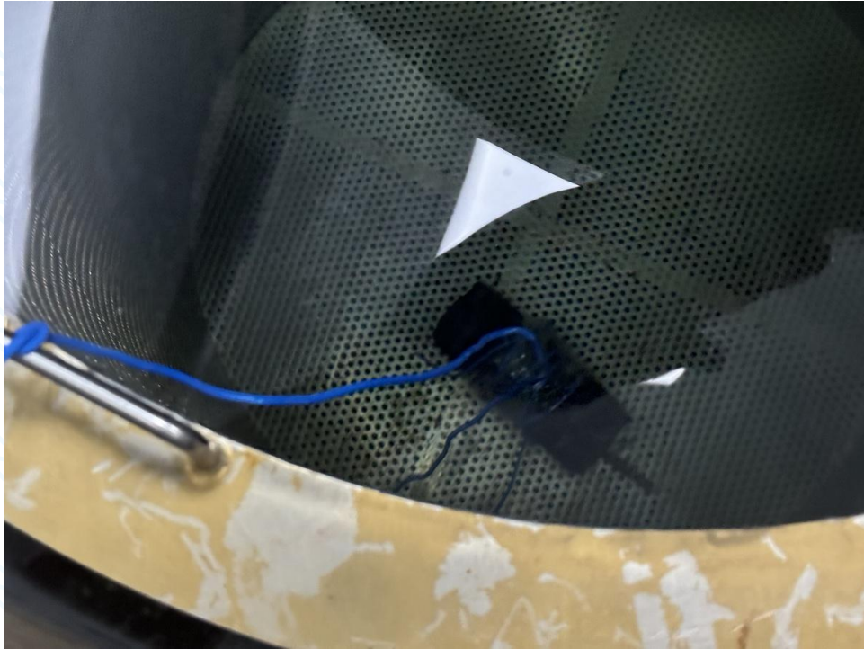
Figure 3: IPX7 test on-going
