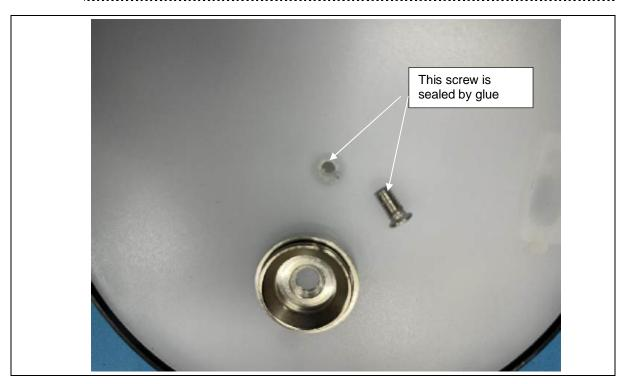
Details of: Base view for TL-RL-1004-3000mAh, TL-RL-1004-2000mAh
