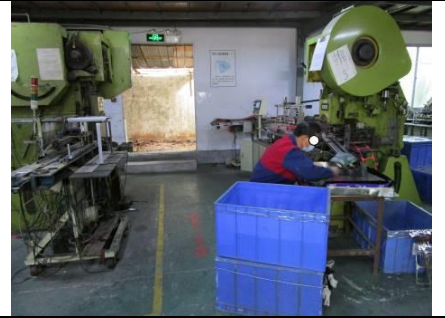
Image 39: One evacuation route in the punching workshop on the 1F of the 2-storey production building was partially blocked by some goods during working hours.
