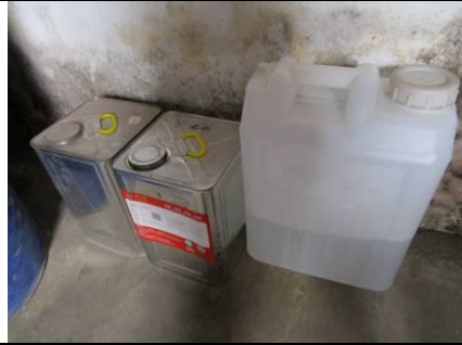
Image 37: No safety labels were marked on two barrels of chemicals.
