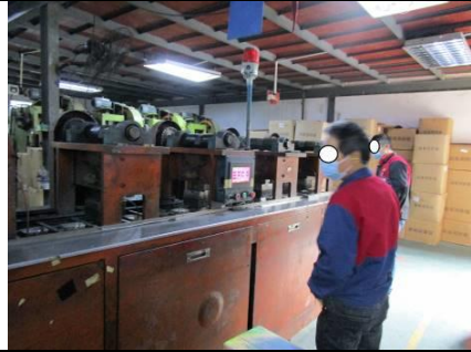
Image 40: One worker in the punching workshop was not wearing the provided earplugs while working.
