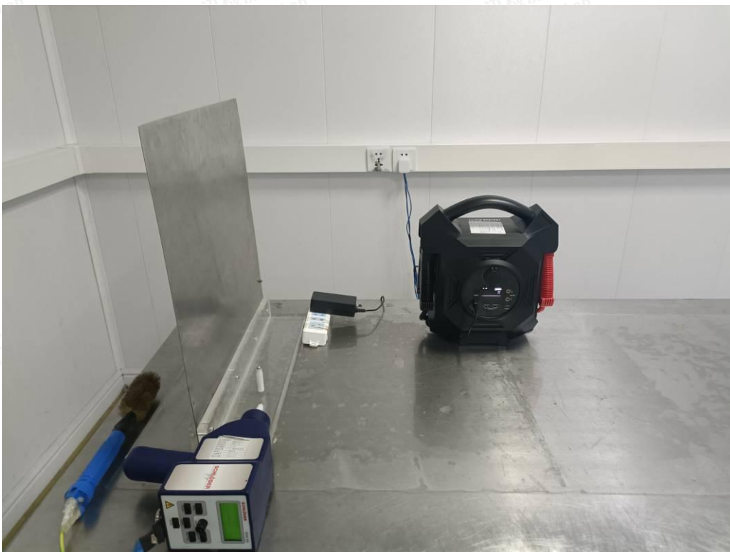
Test Setup Photo of Electrostatic Discharge Test
