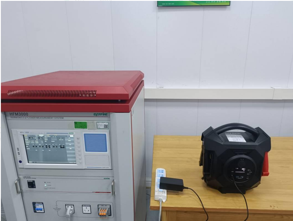
Test Setup Photo of Harmonic & Flicker Measurement
