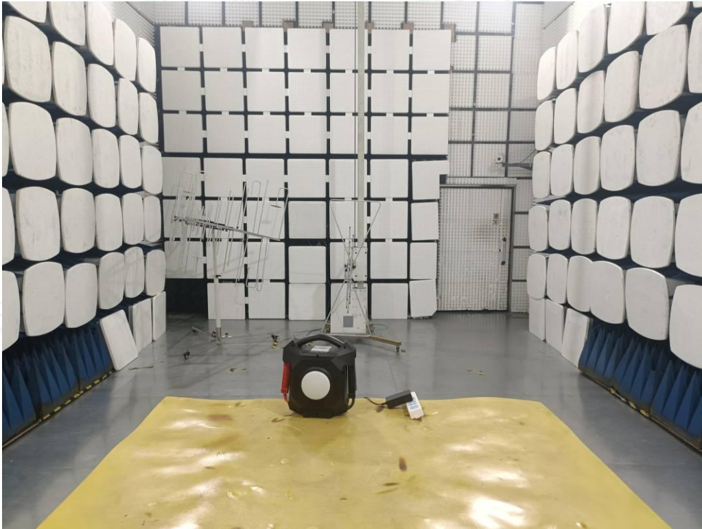
Test Setup Photo of Radiated Measurement (30MHz~1GHz)
