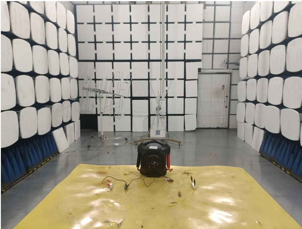
Photo of Radiated emission Measurement(30-1000MHz) (Mode 2)
