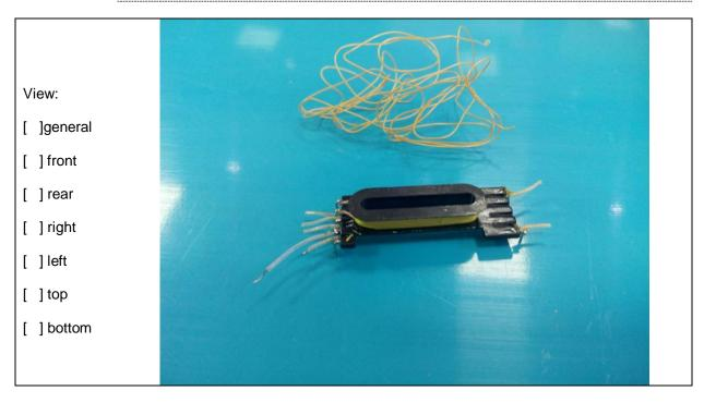
Details of: Transformer, primary winding with insulation tube.
