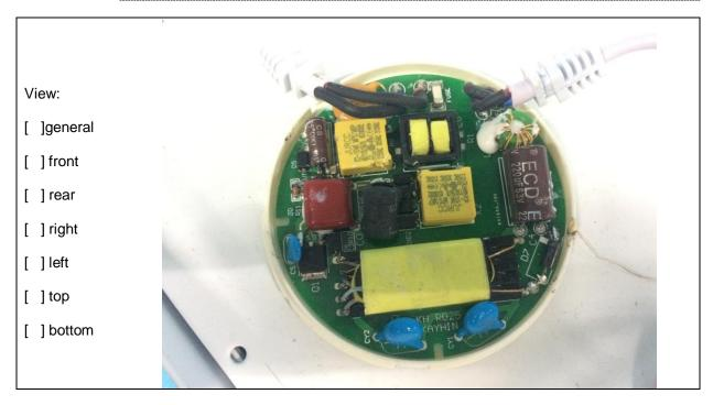
Bottom view of driver PCB Details of:
