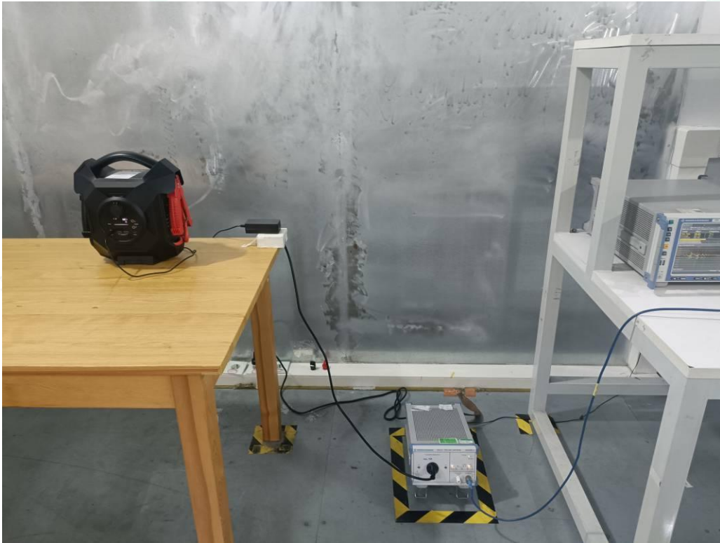
Photo of Power Line Conducted Measurement
