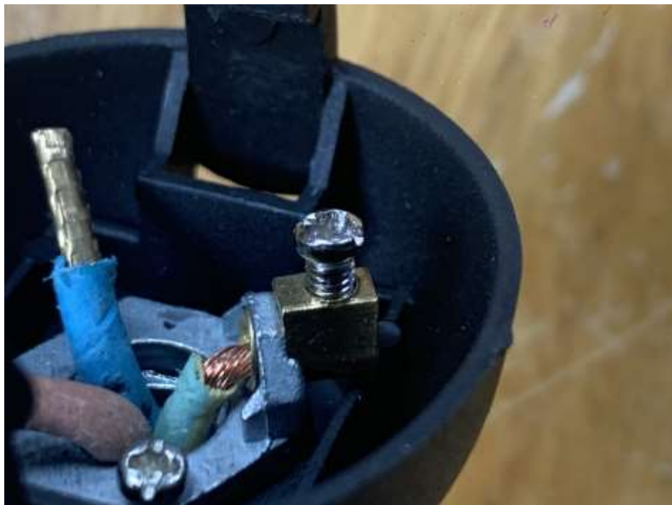
Lampholder internal view and earth wire connection
