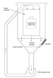
After test, there was no deposit of talcum powder inside enclosures for dust-tight luminaires.
