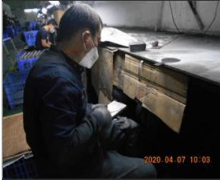
Photo of non-conformity NC no goggle or no cover for rolling part.JPG
