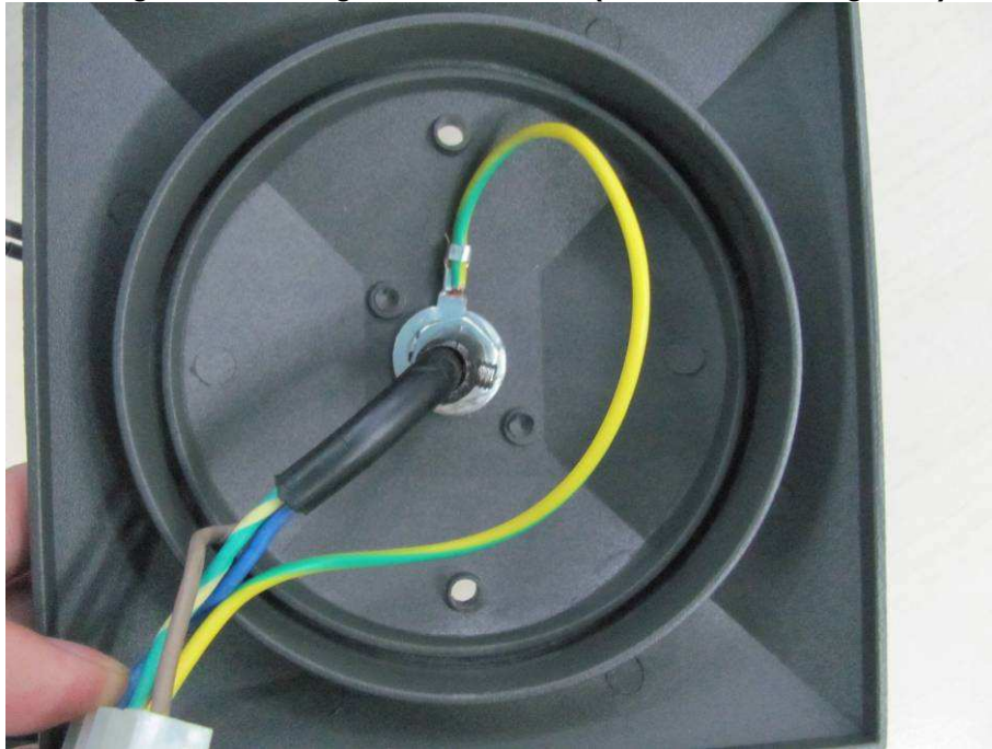
Cord anchorage and Earthing for models ***5 (inside of mounting base)
