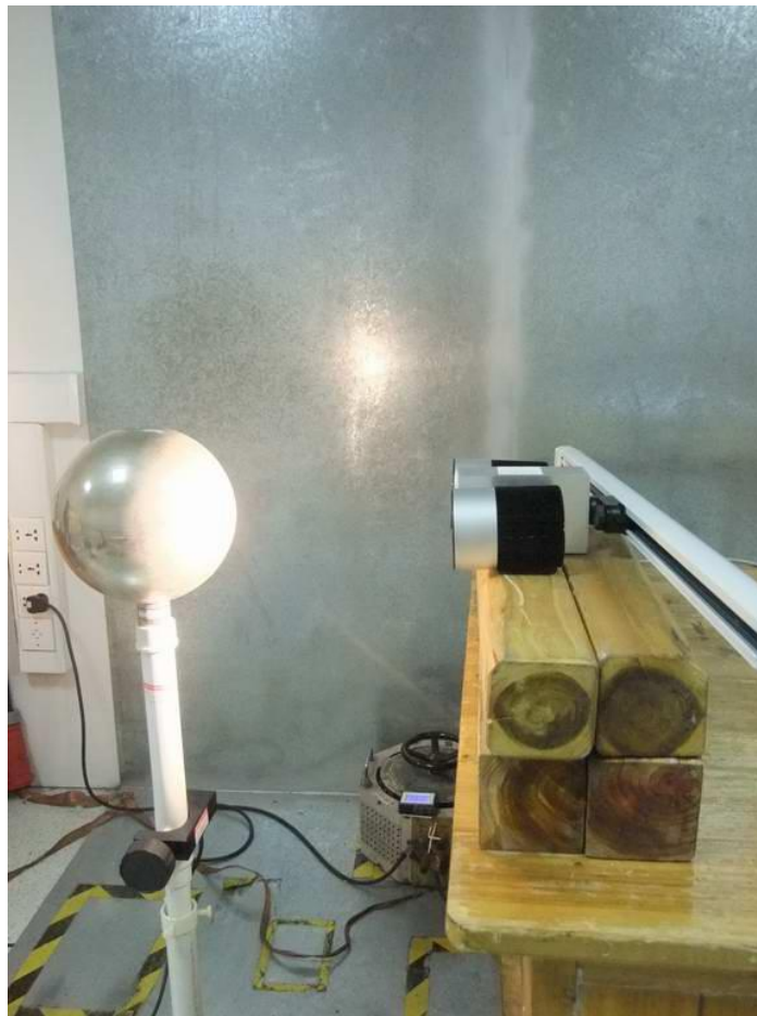
Photograph 1: Set-up for Induced Current Density (20kHz – 10MHz)
