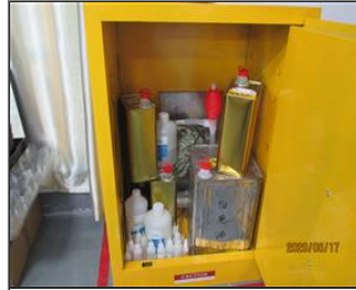
Photo of non-conformity NC 7.7 Thinner missing relevant safety labels.JPG
