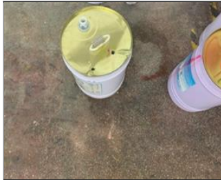
External photo(s) of the production unit(s) NC 7.7 Chemical without safety label.JPG
