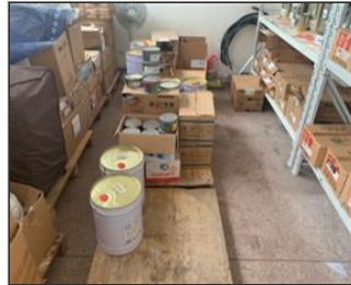
External photo(s) of the production unit(s) NC 7.7 Chemical without secondary container.JPG
