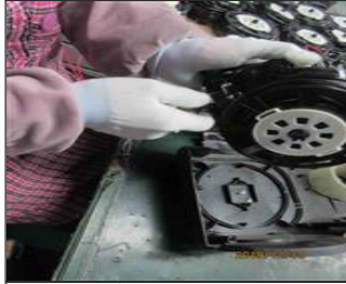
External photo(s) of the production unit(s) 7-6 Did not wear antistatic wrist strap.jpg
