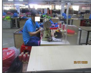
Photo of non-conformity NC 7.17 No pulley guards.jpg
