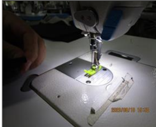
Photo of non-conformity NC-No finger protective guard.JPG
