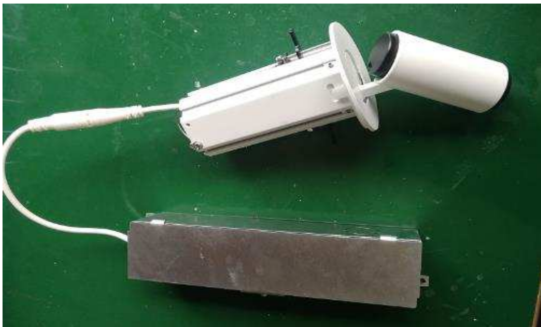
Photo 59a - Alternative structure view of quick connector for VMDL003001A007
