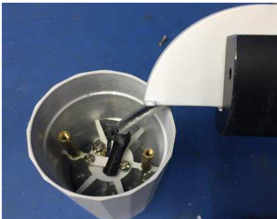
Photo 16 - Grounding terminal view of VMDL004101A008, VMCL004101A008
