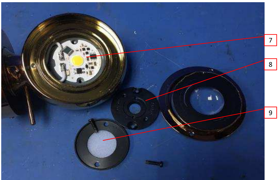
Photo 4 - LED module view of VMWA004201A008
