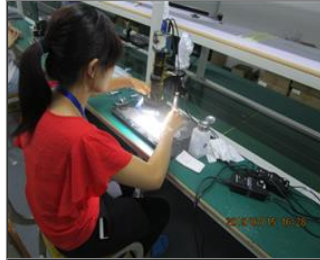
Photo of non-conformity NC Worker use chemical did not wear mask.JPG
